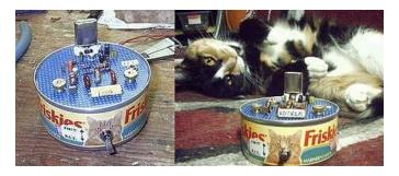
So I figure you have recognized what this is. If not, it is TUNA IN A CAN, or for the rest of the radio people it's a QRP radio in a tuna can. Here is the schematics and the webpage for it. Make and come to the GARS meeting and show it off.
